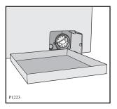
pull out the emergency emptying cap from the filter cover, using a pliers.
